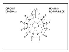
connected to the common, and terminal 1 is open. In position 2, terminal 3 thru 12 and 1 are connected to the common, and terminal 2 is open. Ahoming rotor deck will function for 25,000 mechanical cycles of operation.
