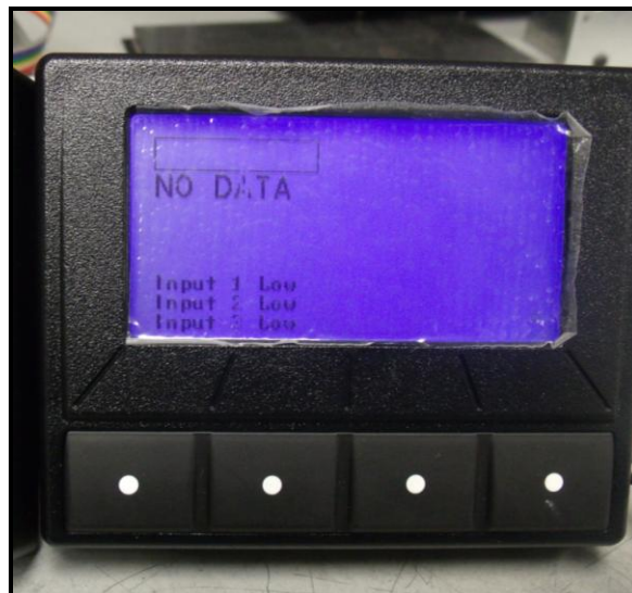
Figure 5—Micro Display after unpowered ±25K
