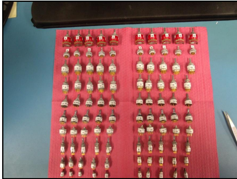
Figure 3– DUT after 48 hours Salt Fog and 24 hours drying (STD plating on the left and NI plating on the right)
