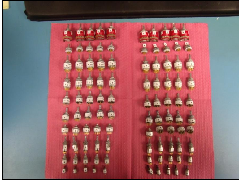
Figure 5– DUT after 96 hours Salt Fog and 24 hours drying (STD plating on the left and NI plating on the right)
