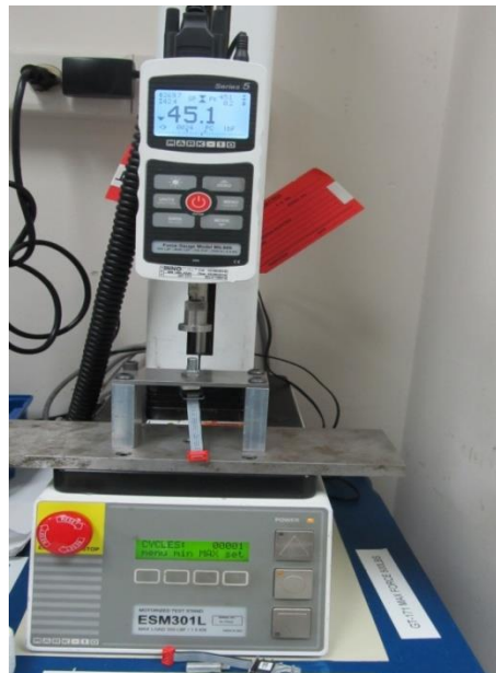
Figure 14 - Push Out Force Test Setup
