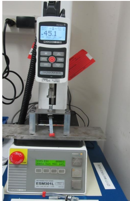
Figure 13 - Pull Out Test Setup
