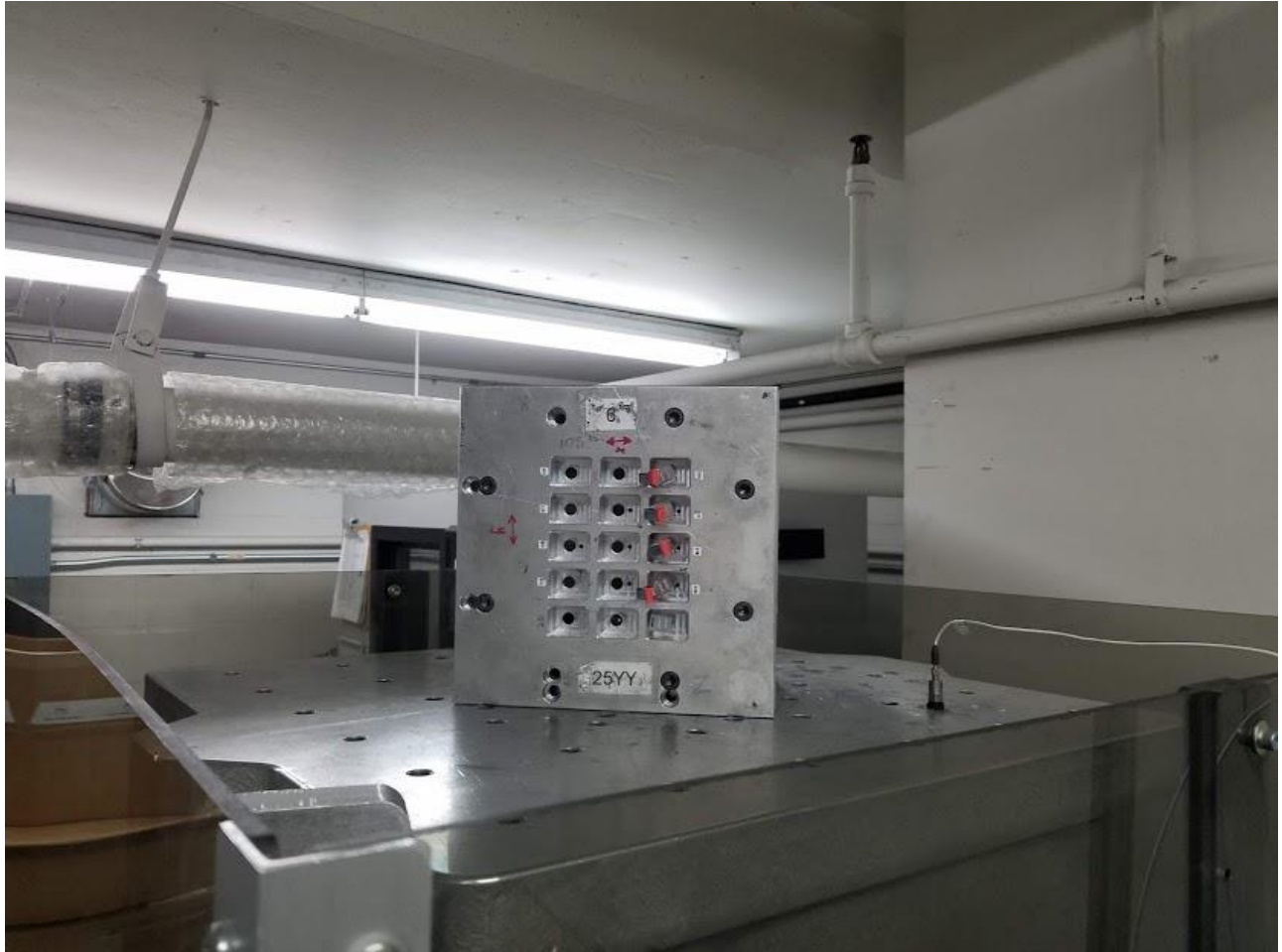
Figure 3 - Mechanical Shock Set-up
