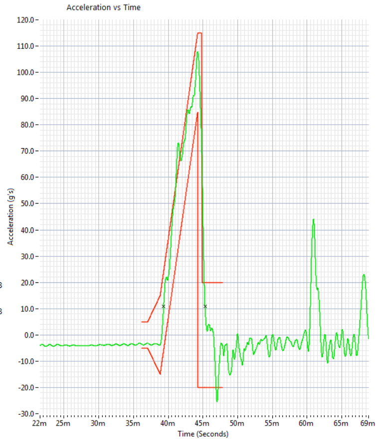
Figure 4 - Mechanical Shock Sawtooth Profile
